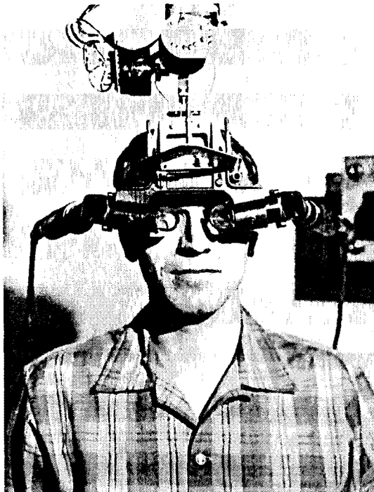
Ivan Sutherland. Front view of user wearing the head-set portion of the head-mounted computer-graphics display system at the University of Utah, 1970. The head-position sensor is shown attached to the head set. The viewer is thus visually surrounded by an imaginary three-dimensional world. Photo by Computer Science Communications, University of Utah, Salt Lake City.
